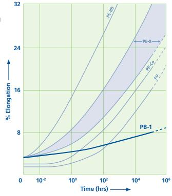
homopolymer form, the balance of properties of PB-1 make it the technically preferred material for the production of pressurised hot and cold water piping systems.
