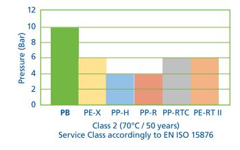
After 10 years of exposure to continuously applied stress, the best performing Polybutene-1 (PB-H & PB-R) retains over 50% more strength than the medium performing materials (PE-X, PP-RCT & PE-RT type II) and 70% - 90% more strength than the lower performing materials PE-RT type I and PP-R.
